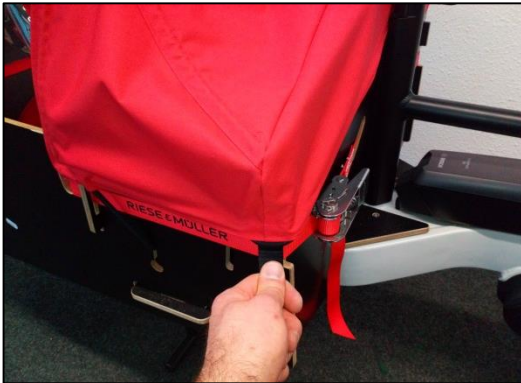
fig. 9: pull cover over side boards
